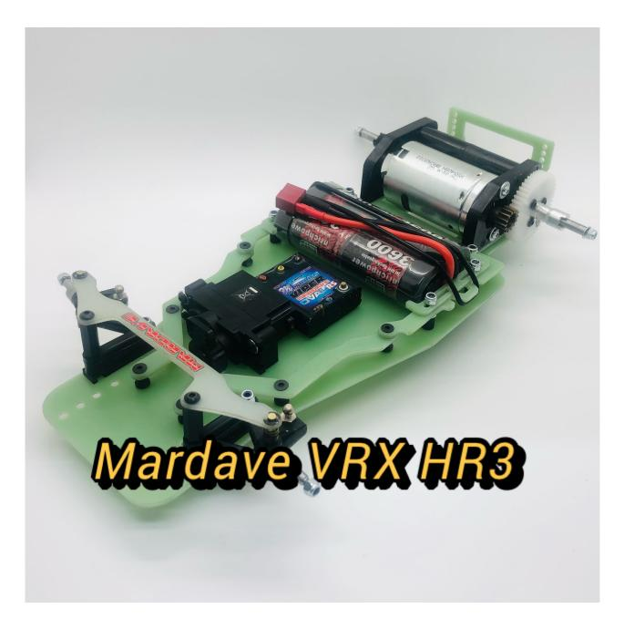
VRX Motor spacer and lowering plate This is used to lower the position of the motor and centralize the motor in the pod
